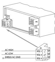
Insert the correct wire in each terminal and tighten the lockdown screw. Tug gently on the wires to verify the connections.
